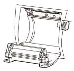
**3** Insert the printer paper in the direction shown below and pull out the paper end to your side by 7 to 8cm.
