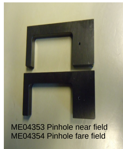
Figure 83: Pinhole for near and fare field adjustment
