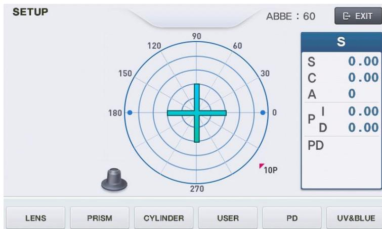
HLM-9000 will start in setup mode. While this mode, 'SETUP' mark will show in the left-upper area.
