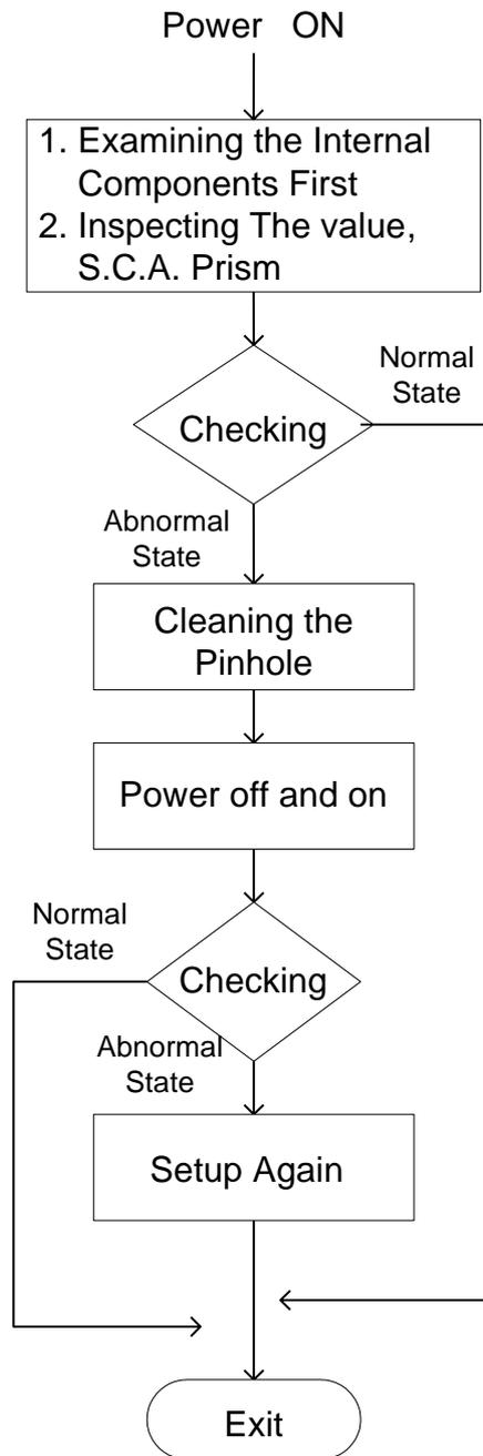
Figure 4. Repair procedure flow chart
