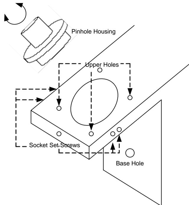
The procedures for changing the Pinhole Housing are as followings:
