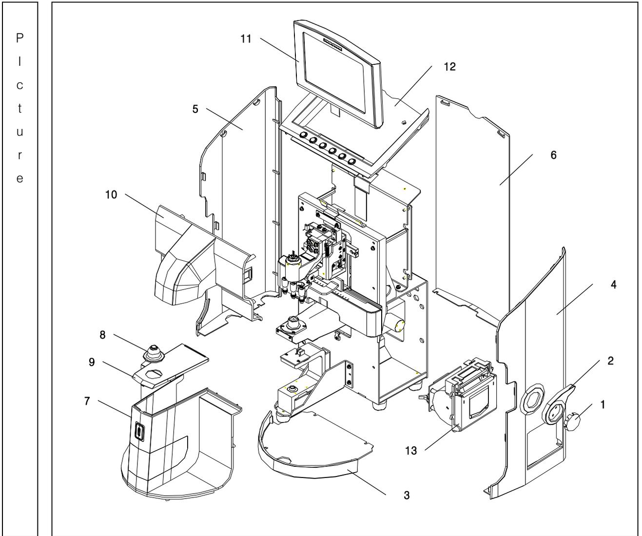
3.2. Disassembling LCD ass'y
