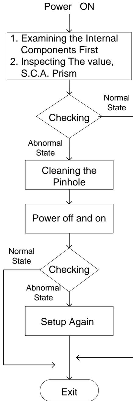
Figure 4. Repair procedure flow chart
