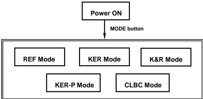
[ Figure 8. Relation between button and measurement mode ]
