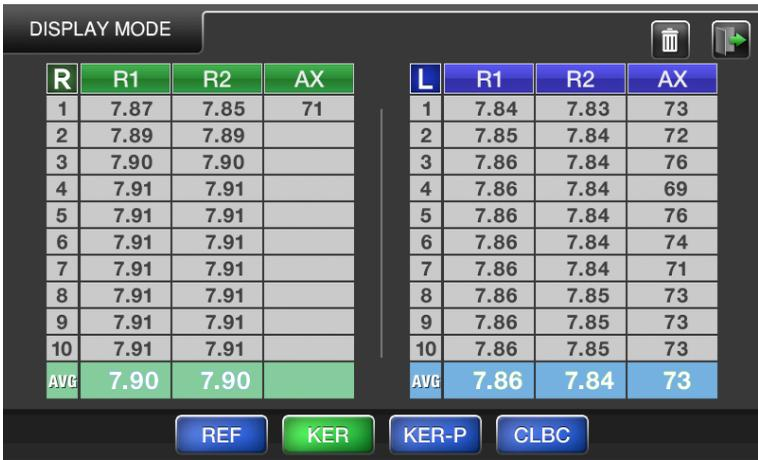
[ Figure 9-6-2. Measured Result of Keratometry, Ker-p, CLBC ]
