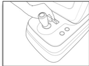
[Figure 7-3. Release of Lock to Stage Section]
