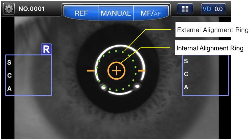
[ Figure 7-4. Adjustment of Measuring Position & Focus ]
