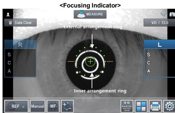
[Figure 6-4. Measurement location and focusing in REF/KER mode]
