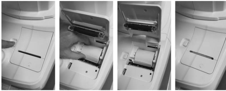
[Figure 9-3-1. Printer paper replacing]
