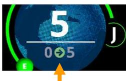
It is possible to choose between counting up and counting down the displayed parameter. The direction of counting is indicated by the direction of the counting arrow on the bottom of the globe.
