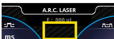
All adjusted values of the posterior applications can be confirmed by taping the blank spot that is located between pulse duration and pulse pause settings or waiting 5 seconds for the device to auto save.
