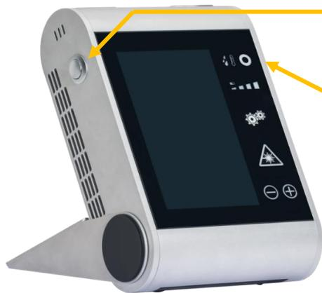
Start the device by long pressing the power button
