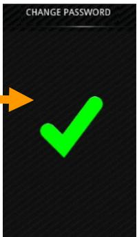
This screen allows to **change the password of the system** that is requested after the startup routine. The password consists of four digits (default is "0000") and the input field is filled by pressing the number keys. After 4 numbers have been entered, the action is completed.
