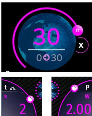
Parameters can be changed by clicking on the corresponding value. The selected value will turn purple and can be adjusted by sliding the point to a different location on the line or by using the plus/minus keys on the side bar.
