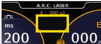
All adjusted values of the posterior applications can be confirmed by taping the blank spot that is located between pulse duration and pulse pause settings or waiting 5 seconds for the device to auto save.
