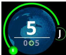
$\mu$ CPC treatment requires the application of a specific amount of energy or a defined laser application time. The counter for these values is located in the center of the display in order to be visible at a glance during the treatment.
