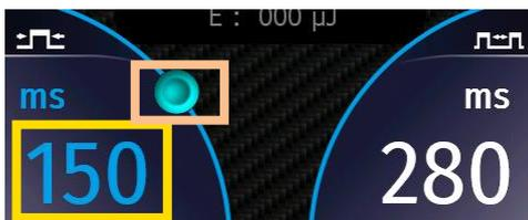
To change the duration of the pulse, presses the current setting. It will turn blue and can be adjusted by sliding the point to a different location on the line or by using the plus/minus keys on the side bar.
