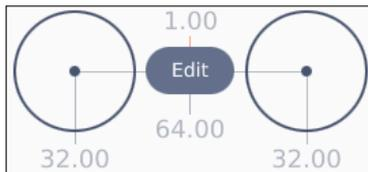
**Pupil distance view:** the two lower extreme values are the right and the left pupil distances. The lower central value is the total pupil distance (right distance + left distance). The higher central value is the vertical displacement between left and right optical points, a negative value means that right points is higher than left point. The distances are expressed in mm. Press Edit to open the pupil distance editor.
