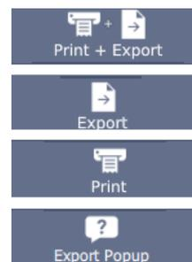
**Output button:** press to Print, Export or Print and Export the measured data. Export Popup allows the user to select a different option each time (see [Chapter 10](#) for details). This button is only enabled after an acquisition.
