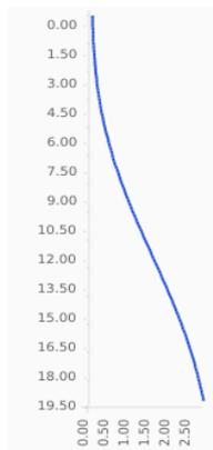
**Addition chart:** it is only available for progressive and degressive lenses. It describes the power profile between the far vision and the near vision points. The x-axis describes the power addition magnitude in diopters, while the y-axis describes the progression in mm from the top to the bottom of the lens.
