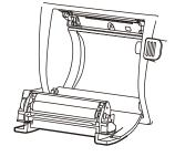
Insert the printer paper in the direction shown below and pull out the paper end to your side by 7 to 8cm.
