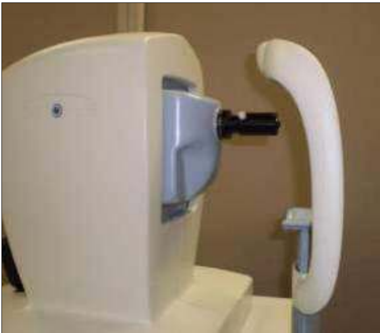
Figure 270 Mounting of Corneal power validation tool
