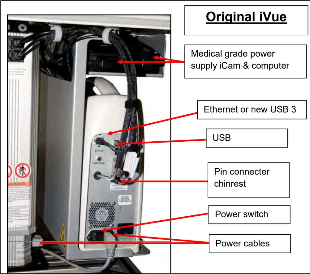
**Original iVue 100 Control Box Cabling Connections**
