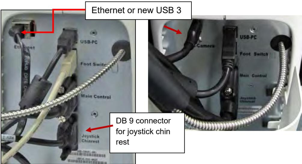
**Current iVue Cabling With DB 9 Joystick Chin Rest Connector**
