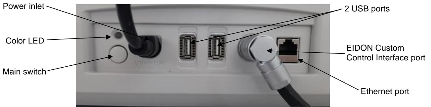
Fig. 6 – Detail of connectors side
