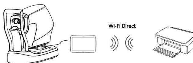
Fig. 82 – EIDON Family device's connection to the printer via Wi-Fi Direct
