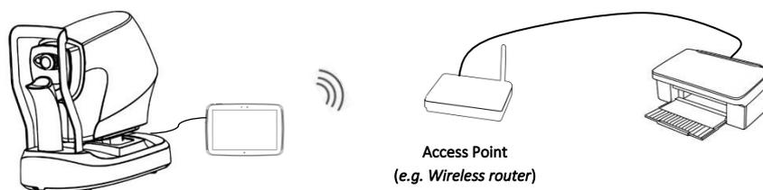
Fig. 81- EIDON Family device's connection to the printer via Access point (cable)
