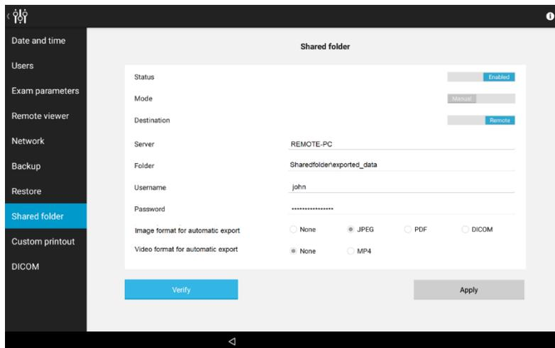
Fig. 98 – Configurator – SHARED FOLDER configuration example: automatic export of JPEG images and MP4 videos to a remote folder *exported\_data* (subfolder of *sharedfolder*), located in the server *REMOTE-PC*, with *John* as server username
