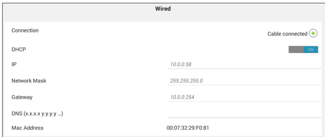
Fig. 90 – Configurator –Network configuration screen
