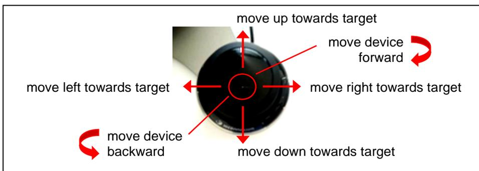
Fig. 39 – 3D Joystick, top view
