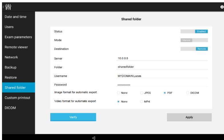
Fig. 99 – Configurator – SHARED FOLDER configuration example, in Windows Domain Networks: automatic export of PDF printouts to a remote folder *sharedfolder*, located in the server with IP *10.0.0.5*, with *Lucas* as domain username and *MYDOMAIN* as domain name
