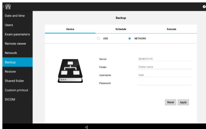
Fig. 93 – Configurator – BACKUP screen – Network backup selected
