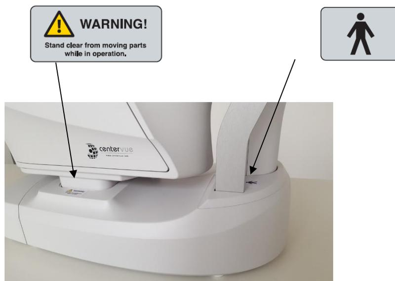
Fig. 9 – Other warning labels on the EIDON Family devices
