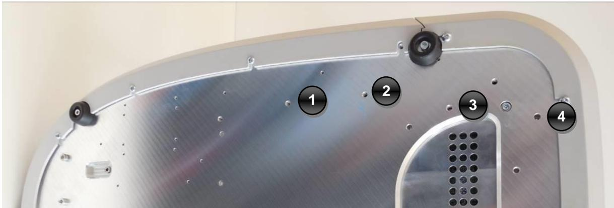
Fig. 15 – Device bottom with holes for tablet and 3D Joystick supports
