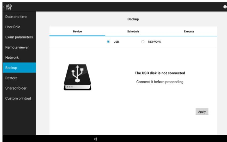
Fig. 92 – Configurator – BACKUP screen – USB-media backup selected
