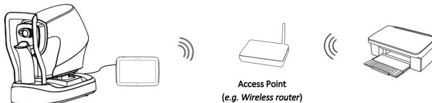
Fig. 80 - EIDON Family device's connection to the printer via Access point (wireless)
