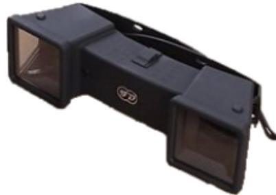
*Fig. 10 – Prismatic stereoscopic goggles*
