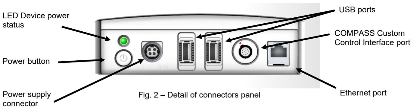
Fig. 2 – Detail of connectors panel
