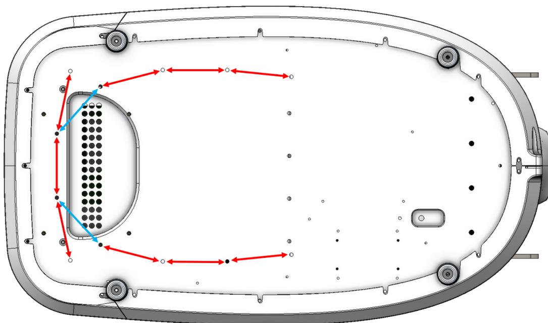
Fig. 10 – Device bottom with holes for the control Interface. Only **RED** positions can be used.
