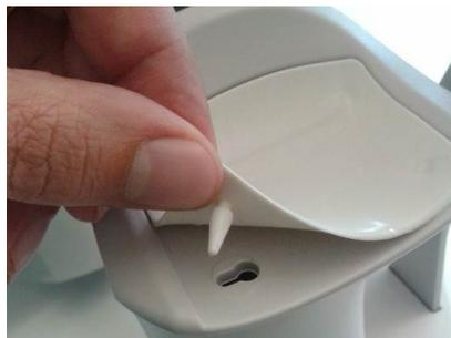
Fig. 97 - Removal of the chin rest silicone pad
