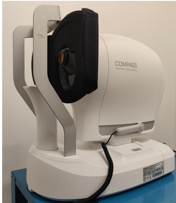
Fig. 11 – Magnetic Light Shield mounted on COMPASS
