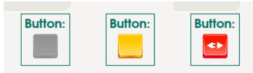
Fig. 26 - Push-button status indicator **on screen** by icon color: *not pushed, pushed, unplugged*
