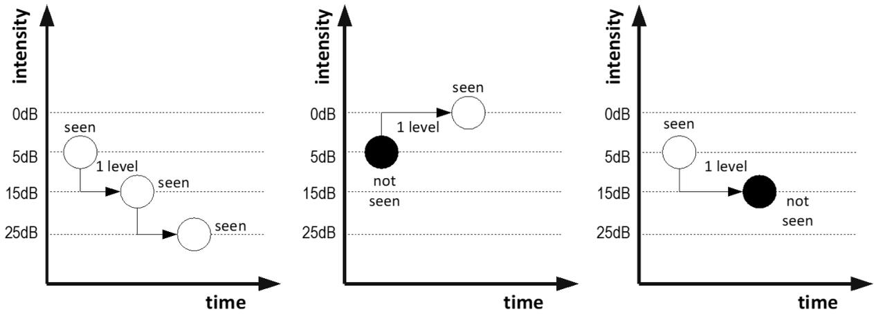
Fig. 24 – Expert test projection logic (4-Levels Fixed strategy)
