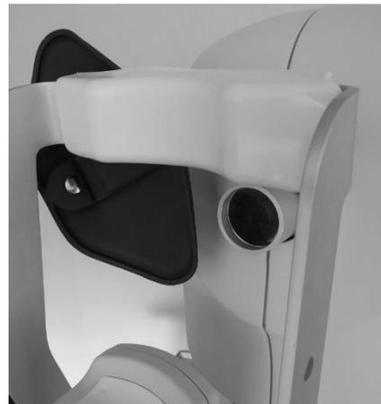
Fig. 13 – Eye Occluder position when examining the right eye
