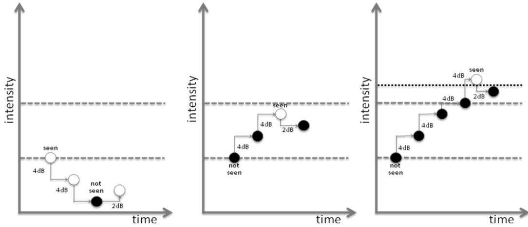
Fig. 23 – Expert test projection logic (4-2 strategy)
